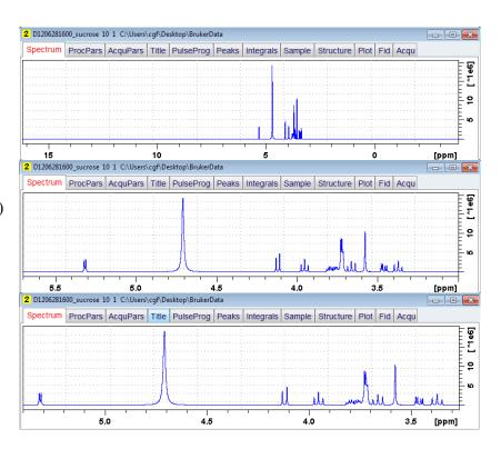
(h) For HSQC (rpar HSQCEDETGPSISP or HSQCETGPSISP) or HMBC (rpar HMBCETGPL3ND), perform step (d) for the <sup>1</sup>H dimension [F2].
