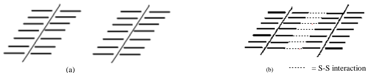
Figure 5. (a) Donor stack interactions in a quasi 1D superconductors (b) Donor stack interactions in a quasi 2D superconductor
